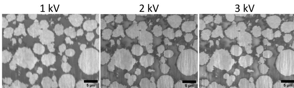
**Effect of acceleration voltage in low-kV SEM:**
