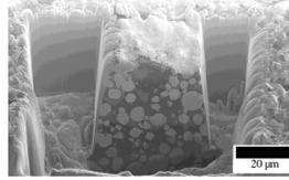
Left: Cross section of li-ion cathode
